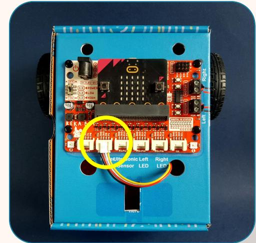
13 Feed the cable through the holes as shown.
