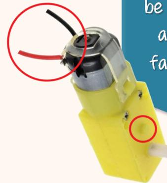
The wires should be facing inwards and the notch facing outwards.
